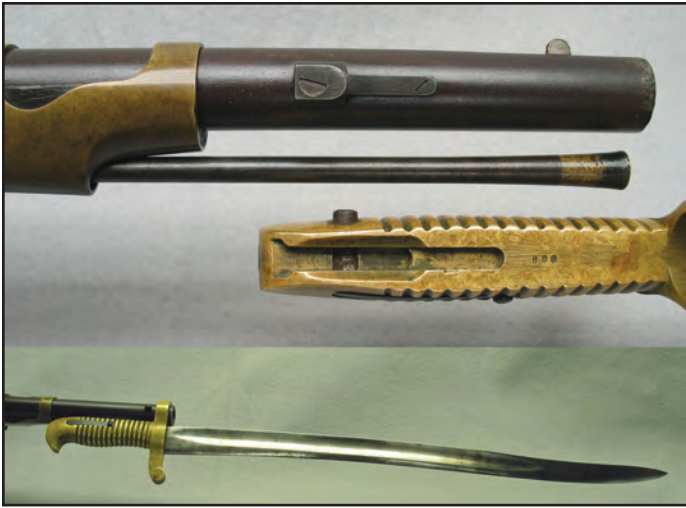
Figure 17. The New Hampshire alteration screwed the bayonet lug and guide to the barrel.
