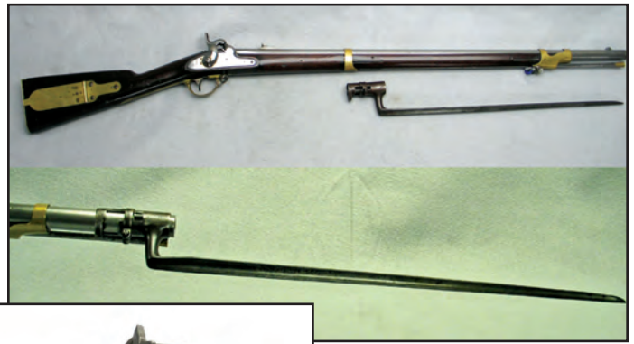
Figure 20. Massachusetts Drake alteration used a socket bayonet.
