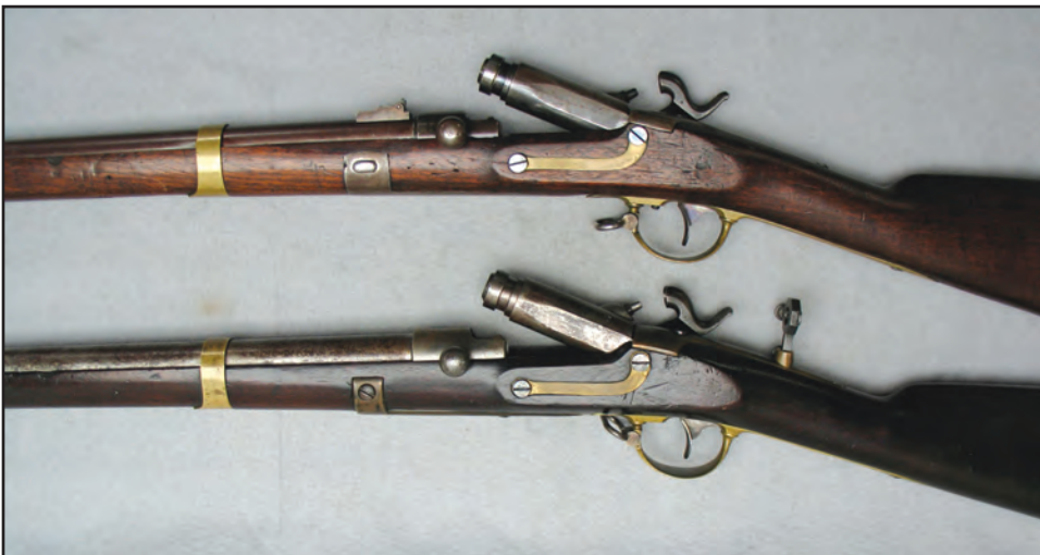
Figure 24. Linder alterations with breech open. Federal alteration on bottom.
