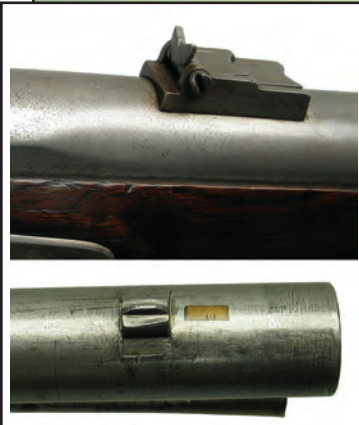
Figure 20. Massachusetts Drake alteration used a socket bayonet.
