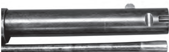
Figure 10. Alterations to muzzle to secure Type I bayonet.
