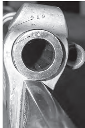
Figure 16. Alphanumeric mating numbers.
