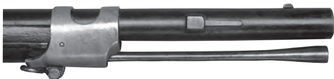
Figure 15. Type II short front band, stud with guide, iron-tipped ramrod.
