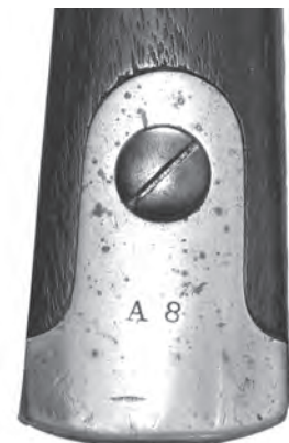
Figure 17. Mating number on tang of butt plate.
